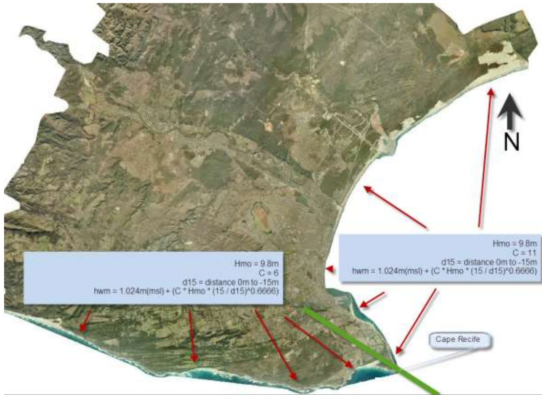
Figure 26 Map of the NMBM coastline divided at Cape Recife and the input parameters for the Mather et al. 2010 formula used to model the HWM
