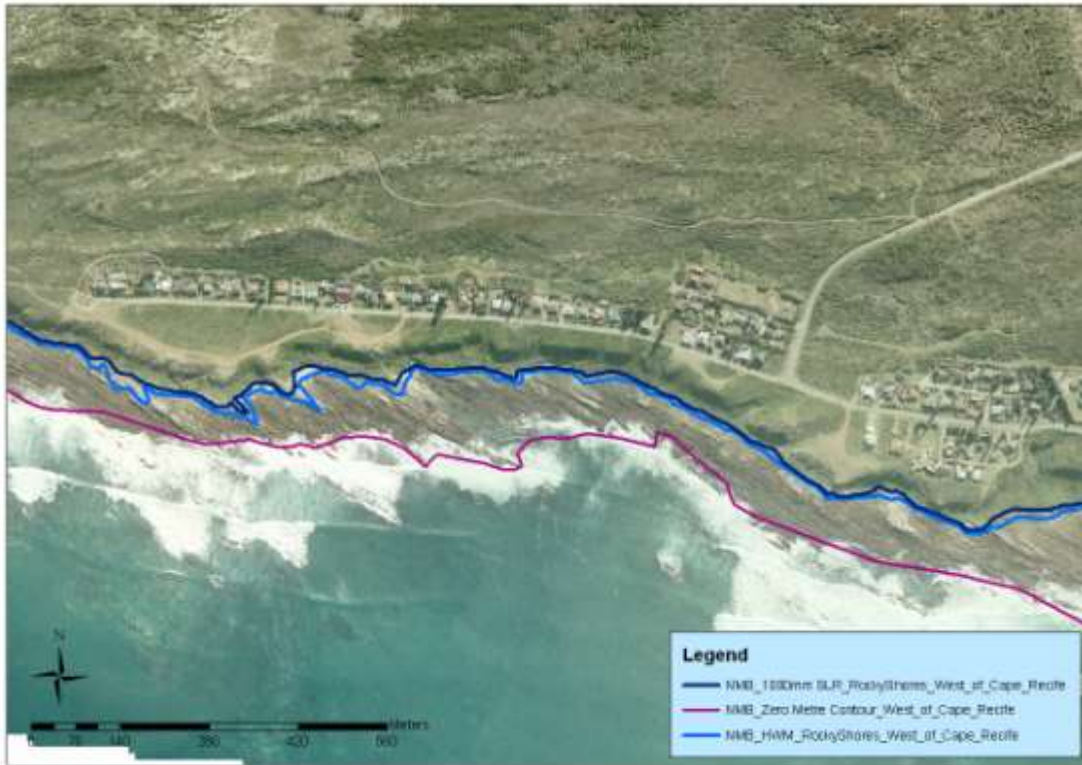
Figure 34 Sea level rise (1000mm) for rocky shoreline area west of Cape Resife.
