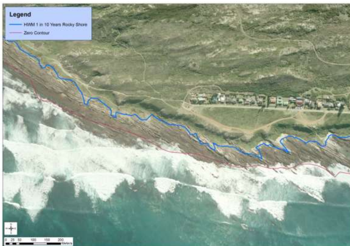
Figure 30: High Water Mark modelling using Eurotop manual for rocky coastline at Schoenmakerskop, west of Cape Recife
