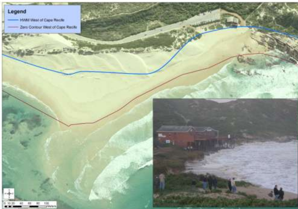
Figure 27: Modelled HWM at Sardinia Bay west of Cape Recife, the results are verified by the insert in the lower right hand corner showing extreme wave run up during the September 2008 storm event, note the position of run up in relation to the two structures.
